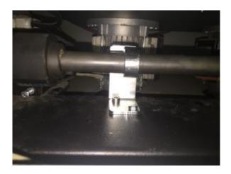
2) When you press the Start button the bar goes down and presses the microswitch at the rear of the hood on the right side (looking from the front). This micro must be pressed about 5 mm before the bar touches the contrast (Silicone/sealing ribbon). You will need to remove the black cover to access this microswitch.
